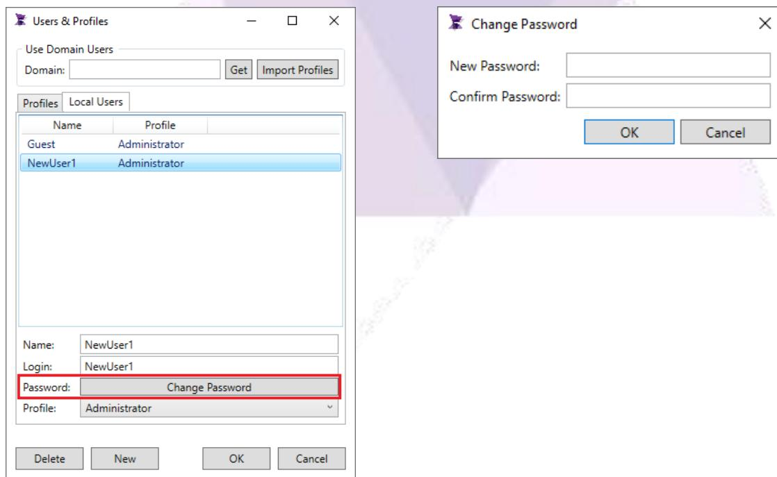
To assign the local user to a profile created in the previous chapter, use the Profile combobox to select an existing profile:
