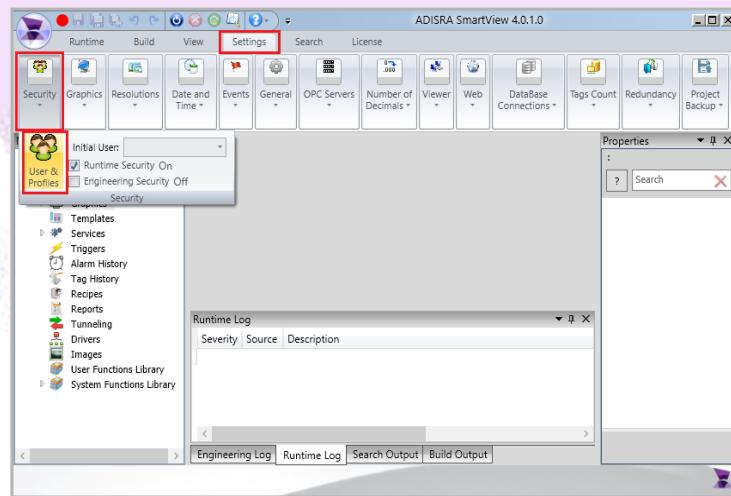
The “Users & Profile” window will open. In the “Domain” textbox, type the domain name of the profiles to be imported, or use the “Get” button to automatically load the domain name where the machine is logged in, then click the “Import Profiles” button:
