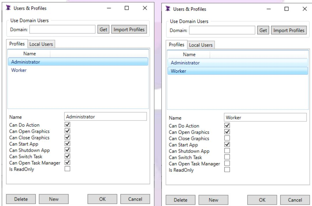
**Note:** When the logged-in user does not have permission to switch tasks, they will not be able to use the machine's operating system while the Viewer is running.
