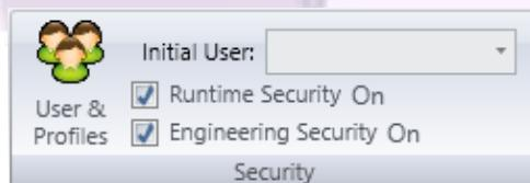
To turn “Engineering Security” off, select the option “Engineering Security” again, and type in the configured password. This procedure will turn “Engineering Security” off.
