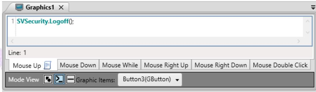
Create a button with the text “Only Admin” and in the button Properties within the “Actions” area, configure as shown in the image below:
